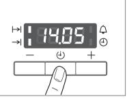
The function indicators Cook time  $\bowtie$  and End time  $\boxdot$  light up and the time is shown in the display. In this example, 12:05.
